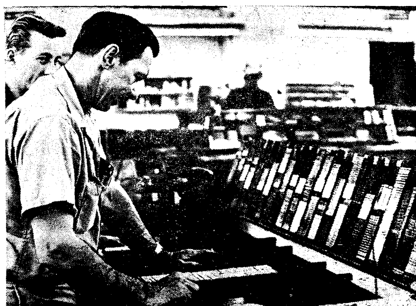
GALLEY PROOFS are made from lines of type, so that corrections may be made and the size of stories may be assessed.
