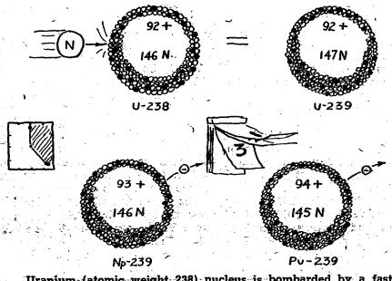
Uranium (atomic weight 238) nucleus is bombarded by a fast neutron, forming U-239. P-239 emits a beta ray (electron) forming Neptunium (atomic number 93, atomic weight 239). The Np nucleus then emits a beta ray and Plutonium is formed.
